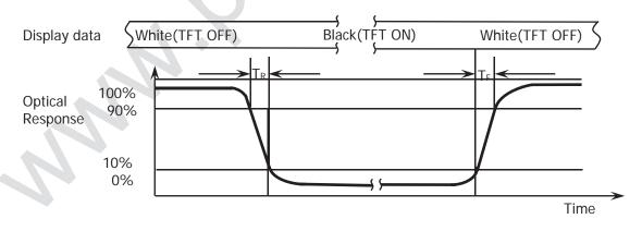
The electro-optical response time measurements shall be made as shown in FIGURE 4 by switching the "data" input signal ON and OFF. The times needed for the luminance to change from 10% to 90% is Td and 90% to 10% is Tr.
