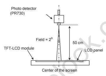
Optical characteristics measurement setup
