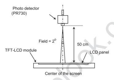
Optical characteristics measurement setup
