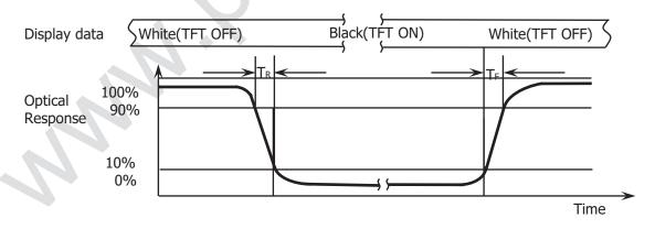
The electro-optical response time measurements shall be made as shown in FIGURE 4 by switching the "data" input signal ON and OFF. The times needed for the luminance to change from 10% to 90% is Td and 90% to 10% is Tr.
