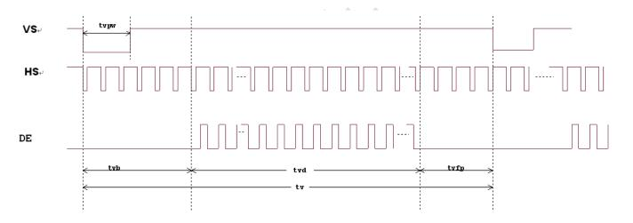
Figure 3. 2 Vertical input timing diagram.
