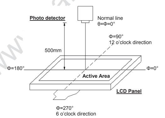
Fig. 4-2 Optical measurement system setup
