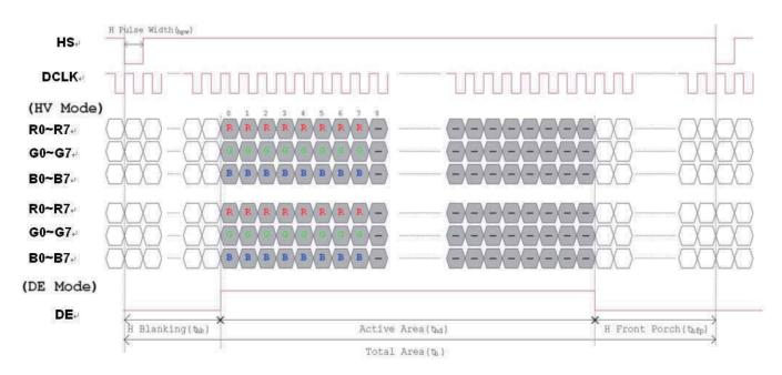
Figure 3. 1 Horizontal input timing diagram.
