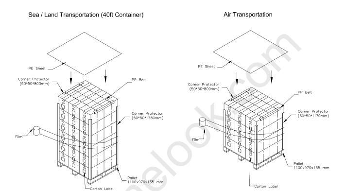
Figure. 9-2 Packing method
