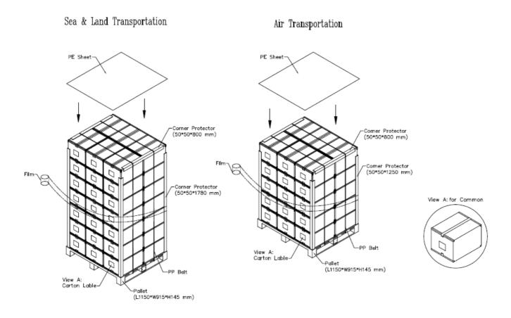
Figure. 7-2 Packing method
