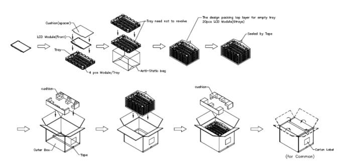
Figure. 7-1 Packing method
