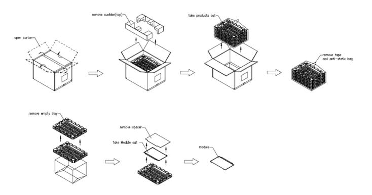
Figure. 7-3 Un-Packing method
