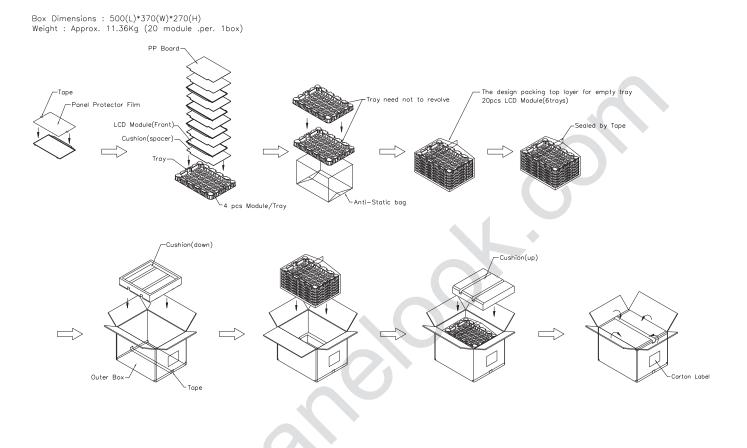
Figure. 7-1 Packing method
