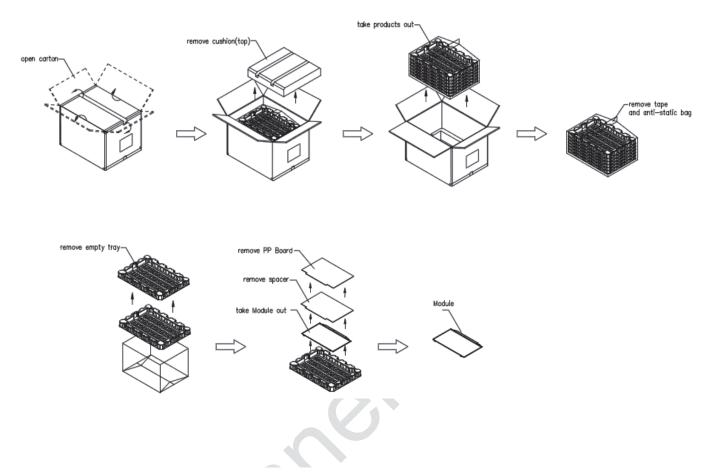
Figure. 7-3 Un-Packing method
